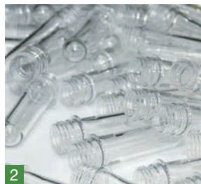
2 Preforms are expanded in a mold and formed into plastic bottles.
