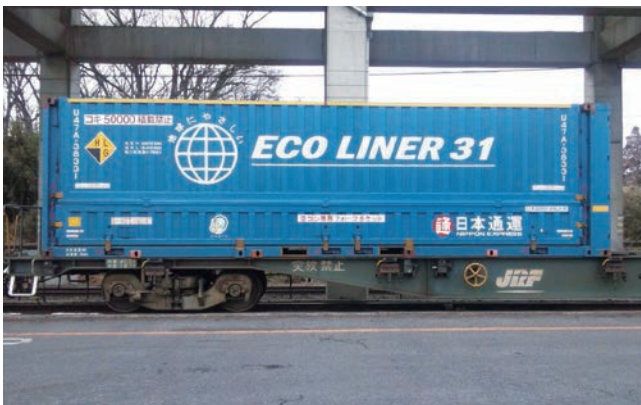
Eco Liner containers that can be loaded directly onto rail transport
