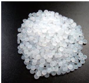
Recycled pellets made from polyethylene scrap
